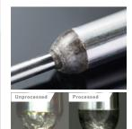
of a few millimeters called the whisker may be generated from the tinning of the lead terminal Whiskers grow larger in time, and short-circuit the electronic circuit or wiring, causing the device to malfunction. We established a unique method for applying UV resin coating to the welded part of the lead terminal and achieved complete elimination of whisker generation
