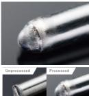
In the assembly process for aluminum electrolytic capacitors, here are some cases where the tip of the lead terminal accidentally contacts the aluminum case and results in a damage, and it has become more and more difficult to nsert it into the small opening on the sealing rubber. We contribute to reduction in the
